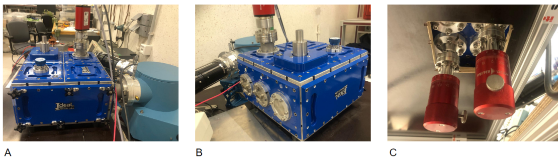
Figure 3.2: (a) Right-side view of the vacuum chamber with the monochromator being the light blue object attached to the chamber. (b) From left to right the pressure sensor, the liquid nitrogen trap and the vent valve. On the left side plate the two D-sub connectors are visible. (c) Cutout in the setup table below the vacuum chamber that creates space for the rotary feedthroughs that control the sample holder and SiPM holder.
