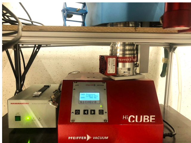
Figure 3.11: Photograph of the Pfeiffer vacuum HiCube 80 Eco DN63 pumping station in the VULCAN setup
