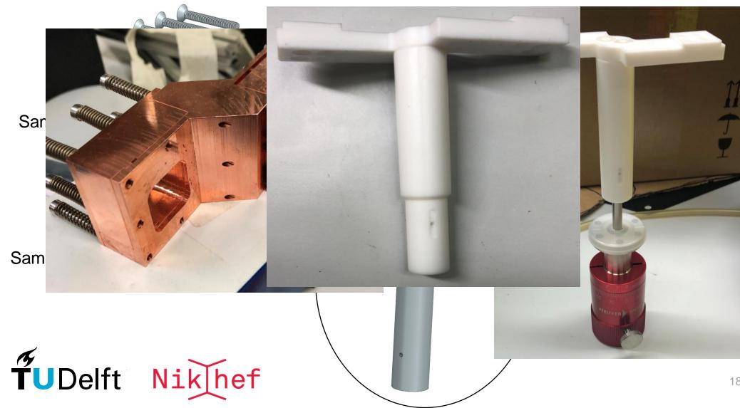
The design and fabrication of the sensor holder
