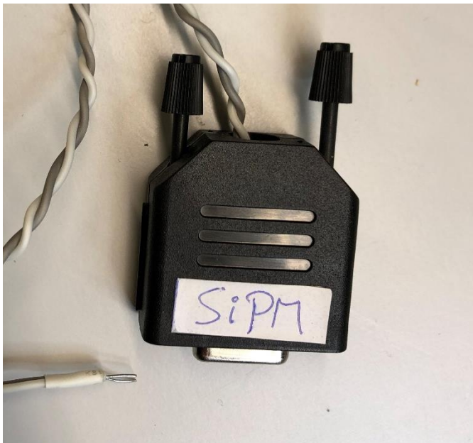
Figure 3-25: The initial set of wires for the connection of the SiPM to de data acquisition. On the left the connector and wire for outside the vacuum, and on the right the wire for inside the vacuum.
