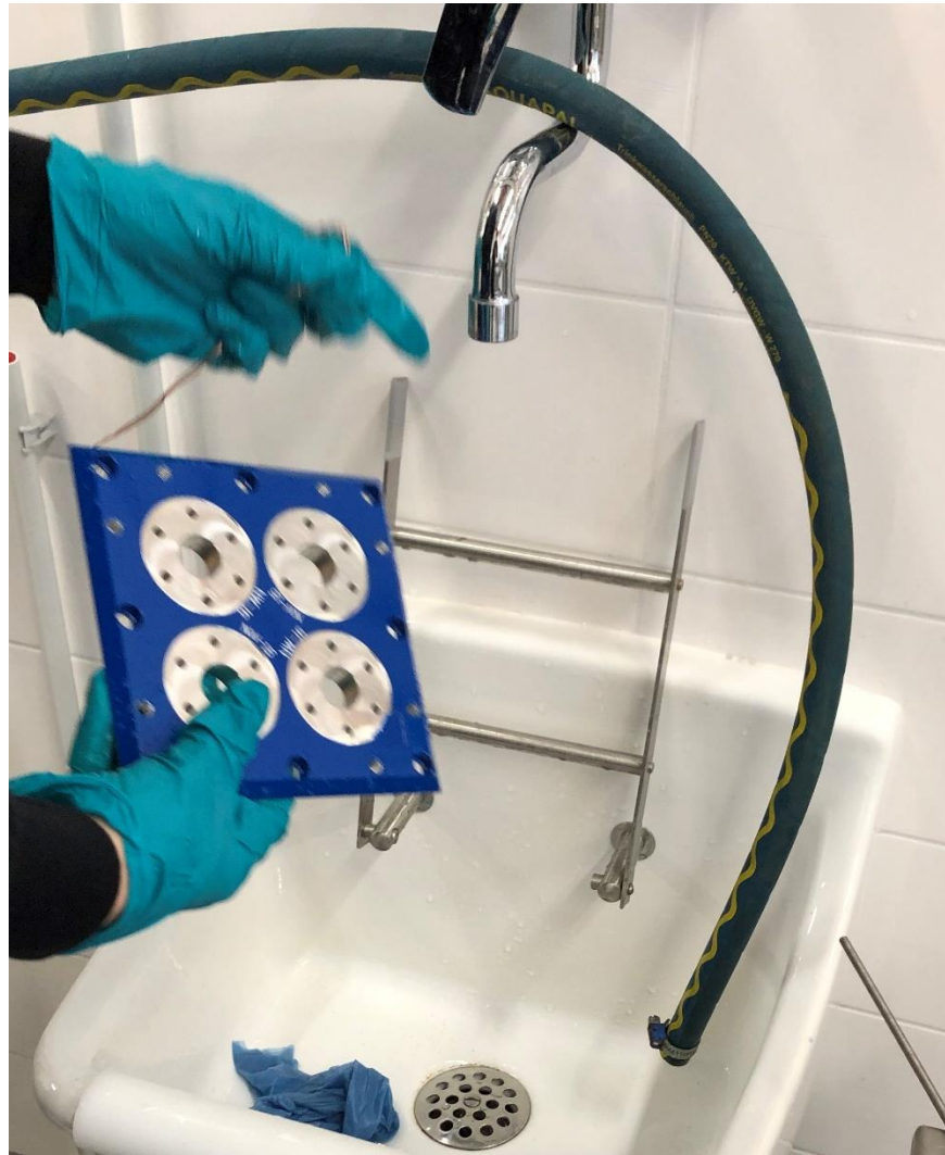
Figure 3-30: The rinsing of the ultrasonically cleaned parts with demi water, to remove any soap residue left on the parts after the cleaning process.
