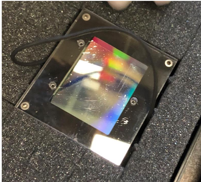
Figure 2-8: Reflective grating covered by protective plexiglass in its storage container. This is one of the most delicate parts of this setup. It can lose its very precise reflective properties if any material settles on its surface.
