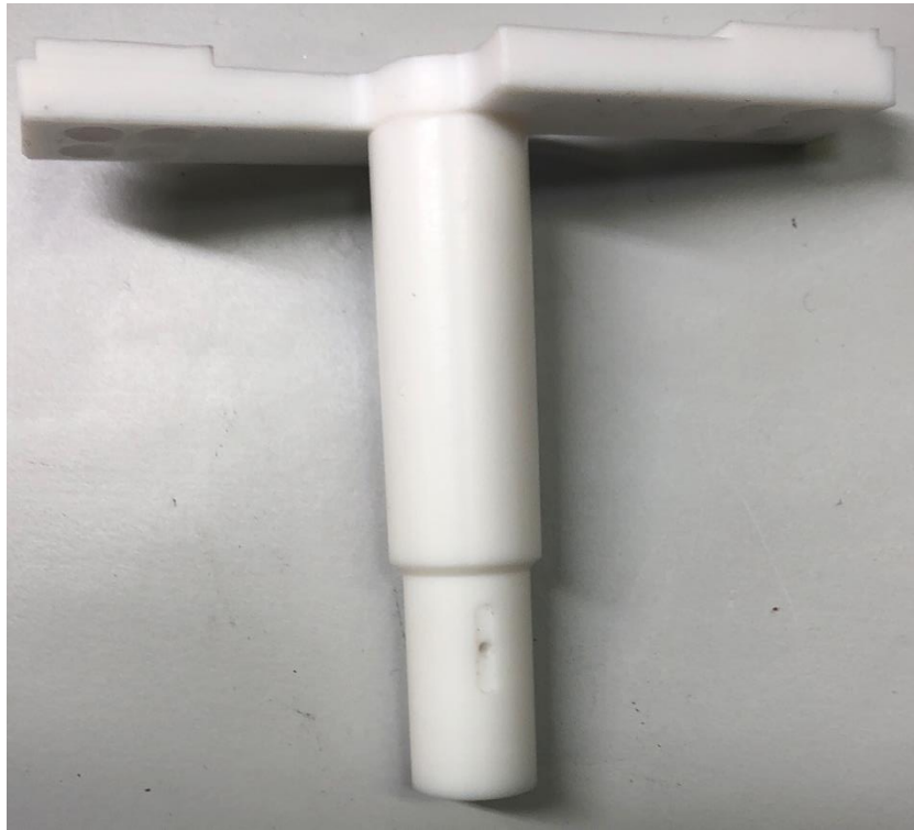
Figure 3-8: The sample holder mount fabricated, assembled, and adjusted to fit the sample chamber.
