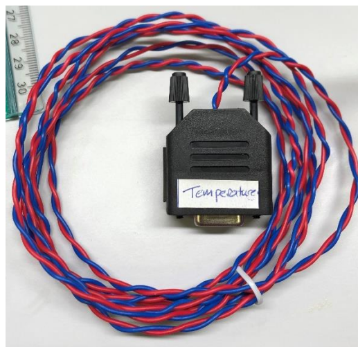
Figure 2-20: Cabling used on the outside of the sample chamber, a connector is used for ease of connection and neatness.
