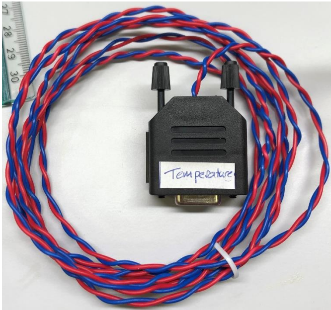
Figure 3-24: The fabricated cables as used outside of the vacuum. On the left an overall view of the twisted pair cable, and on the left a zoomed picture of what the connector looks like.
