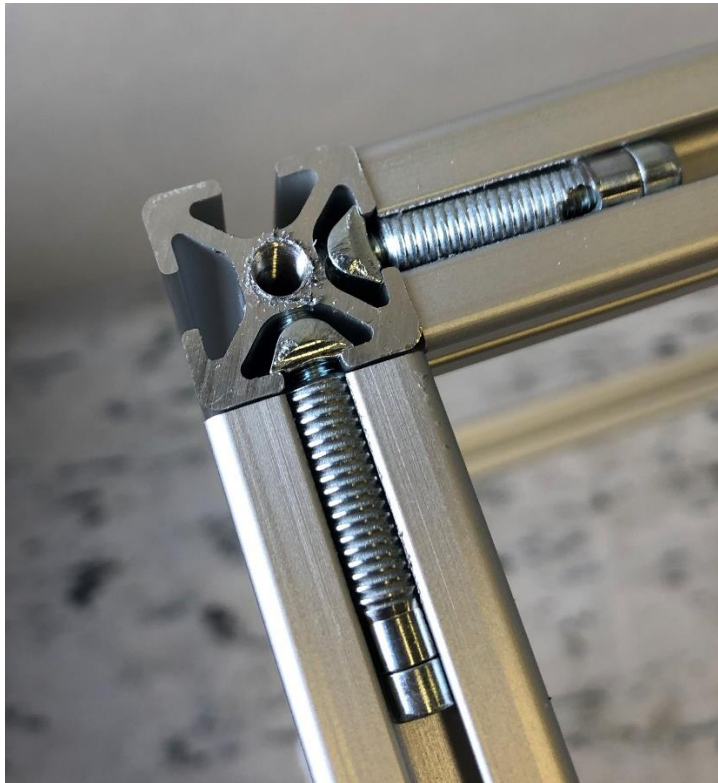
Figure 3-14: The profile 5 beams of 20 x 20 [mm] with the original fasteners. In the image is visible how this looks like when all is installed.
