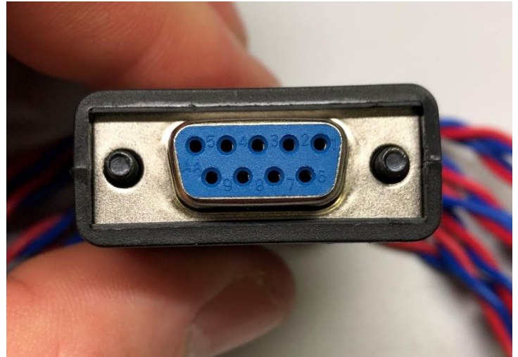
Figure 3-24: The fabricated cables as used outside of the vacuum. On the left an overall view of the twisted pair cable, and on the left a zoomed picture of what the connector looks like.
