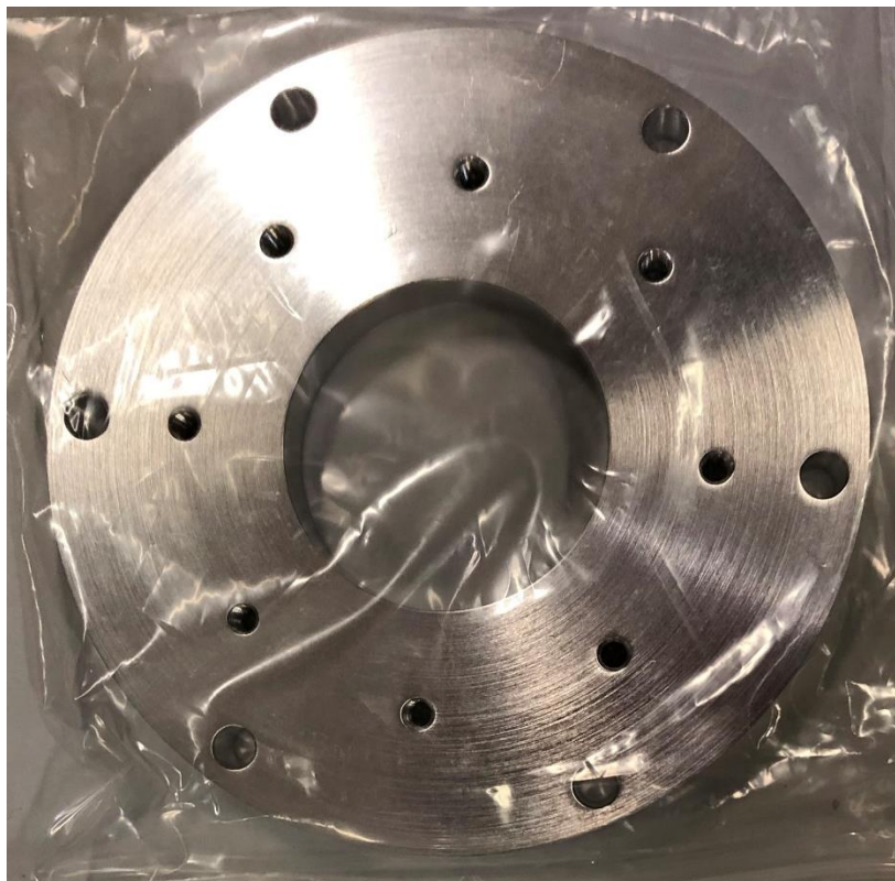
Figure 3-26: The original adapter made by McPherson. This adapter will enable us to connect their in-house nonstandard flange to the standardized KF flange on the vacuum chamber.
