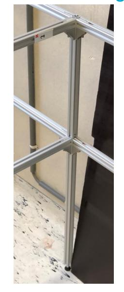
Adjustments made to the setup table to ensure its rigidness with the experiment placed on it.
