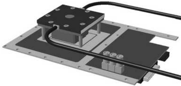
Figure 3.1: DICE setup. On the left the chamber is visible, with cables coming to and from it for the injection and outflow of the gas. Below on the right the connector for the Muros data acquisition device is shown [7].
