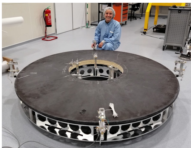
Figure 2: Stiffening disk on the aluminum support frame, during the sensors installation. This happened before moving everything into a box where the temperature was controlled.
